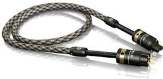
They are 100% shielded against distortion due to a 2-layer ALU/PET shield (aluminum foil sheets) and the inner core is made for tinned braided OFC screen (32x 0.10) GS 3x silver plated OFC copper strands.
